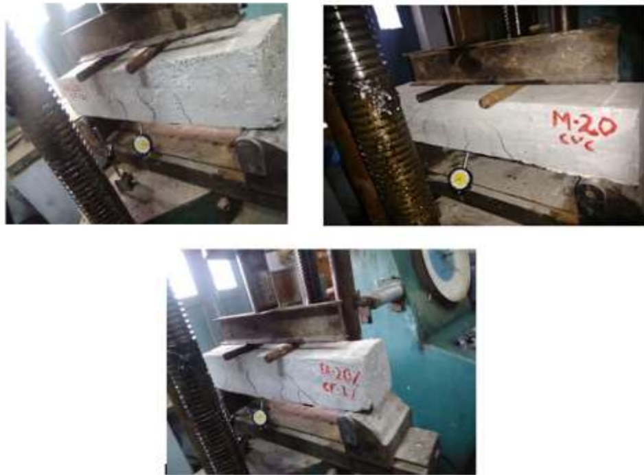
Fig 6: Crack Pattern Of Test Beam
